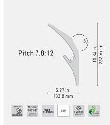
The **ARCUS** moulding is designed for slanted surfaces, such as in **attics or cathedral ceiling rooms**. It levels out flush with 1/2" or 5/8" gypsum panels, and contains a recessed LED channel for smooth lighting of the ceiling perimeter. Fits most common slant angles, with room for adjustment using drywall mud. It can be primed and painted like a regular wall surface.
