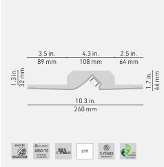
The LATUS is an asymmetric recessed LED moulding for drywall, allowing washing an adjacent surface with light from a 45-degree angle, from a distance of your choice. The uniform light distribution enhances the appearance of art and displayed items. A direct fit with standard gypsum panels, it needs only a low (1-1/4in.) back clearance, and can be easily installed between smaller beams or joists.
