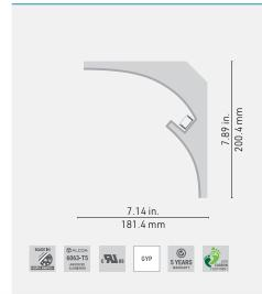
Smooth out those corners with a **rounded light extravaganza!** The APSIS will go into any corner, whether wall or ceiling, and level out flush with the 1/2" gypsum panels. Prime and paint, mount the aluminum LED profile with your choice of lens, and breathe a brand new life into your interior. As easy as it gets!
