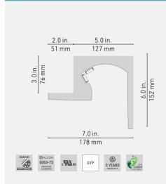
The **NIDUS** profile is an easy and affordable solution for lightgrazing a wall, while keeping the LED source concealed and the corner visually intact. Install over 2×3in. beams/joists, without the need to build elaborate wood structures, level with the gypsum panels, then mount the LED profile(s) at the position yielding the desired beam direction. Great above blinds or curtains!
