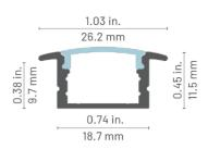
The 1300 profile is designed for recessed linear lighting applications. The 1300 profile offers a wide selection of lenses, light outputs, and color options to produce a uniform linear light housed within a channel of extruded aluminum. The flanged edges of the extrusion add a decorative trim for a discreet and clean recessed appearance.
