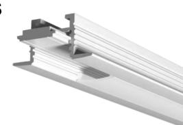
The 1500 profile is designed for recessed linear lighting applications. The support rail accommodates type B joiners to connect multiple sections and to go around corners and from wall to ceiling. The 1500 profile offers a wide selection of lenses, light outputs, and color options to produce a uniform linear light housed within a channel of extruded aluminum. The flanged edges add a decorative trim and can be easily installed with a spring bracket.
