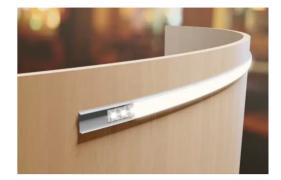
The 5560 profile allows integrating linear LED lighting on curved or uneven surfaces. Its low profile (1/5" including lens), and a thickness of less than 1/32" (0.75mm), allows for effortless bending and installation using plain mounting tape or screws. The opal lens will provide a diffused light effect without harsh dots.
