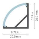
The 2000 is designed to allow extra lighting angles. The profile can be installed to project at 30 or 60 degrees, two angles for lighting extra deep or high scenes, to bring out the finest details, without hot spots.
