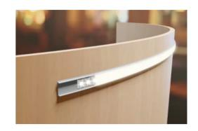
The 5560 profile allows integrating linear LED lighting on curved or uneven surfaces. Its low profile (1/5" including lens), and a thickness of less than 1/32" (0.75mm), allows for effortless bending and installation using plain mounting tape or screws. The opal lens will provide a diffused light effect without harsh dots.
