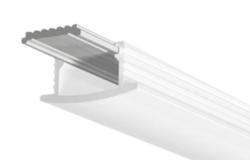
The 5100 consists of an aluminum heatsink base inserted into a flexible recessed lens with gripping sides. It allows for a very simple installation, with the assembly inserted into the recess and staying in place due to the gripping ribbed lens sides. The 5/8" wide and 3/8" deep recess is a direct fit for North American cabinetry, closet, or mural applications, besides being economical and providing lighting without hot spots.
