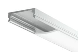
This profile is the thinnest of the 1000 series being only 6mm thick and 18.7mm wide and is compatible with most of our LED strips. Perfect for tight spots, it will be very discreet and will stand out.
