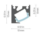
Our range of ultra-compact profiles has been expanded! The 4200 profile provides accent lighting at an angle of 30° to highlight products on shelves or to cut out the underside of cabinets. A notch on the underside completely conceals the TR64 mounting wire, giving the luminaire an even more aesthetic look. Ideal for commercial or residential applications.
