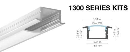
The 1300 profile is designed for recessed linear lighting applications. The 1300 profile offers a wide selection of lenses, light outputs, and color options to produce a uniform linear light housed within a channel of extruded aluminum. The flanged edges of the extrusion add a decorative trim for a discreet and clean recessed appearance.
